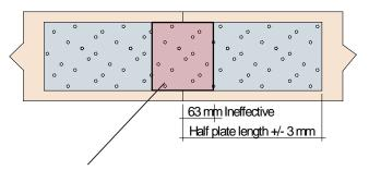
Nails in this ineffective region (close to end-grain of timber) must be avoided to prevent splitting.
